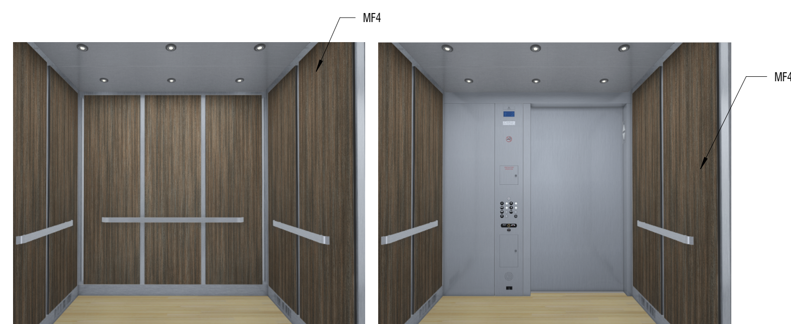
A1 ELEVATOR CAB FINISHES
